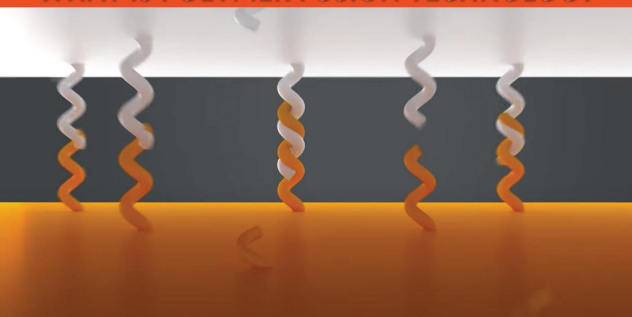
The merging of two separate polyolefin thermoplastic polymers together (polymer fusion label + polyolefin product) using melt-point, time, and pressure to produce a singular piece of plastic without adhesives, tie layers, bonding agents, or use of secondary surface treatments.
