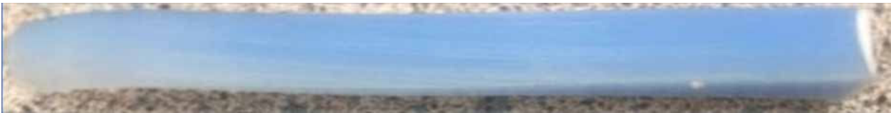
Figure 1: Side Wall Bubble Free - Perfect Cure at 12% cycle time reduction
